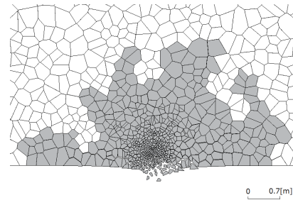
Fig. 9 Fragmentation around the blasthole (burden=0.425m)
