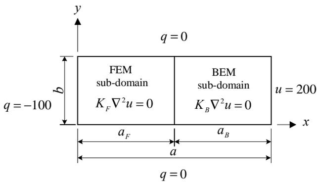
Figure 3: Potential Flow Problem with Neumann Boundary Conditions Specified on the Entire External Boundary of the FEM Sub-domain.
