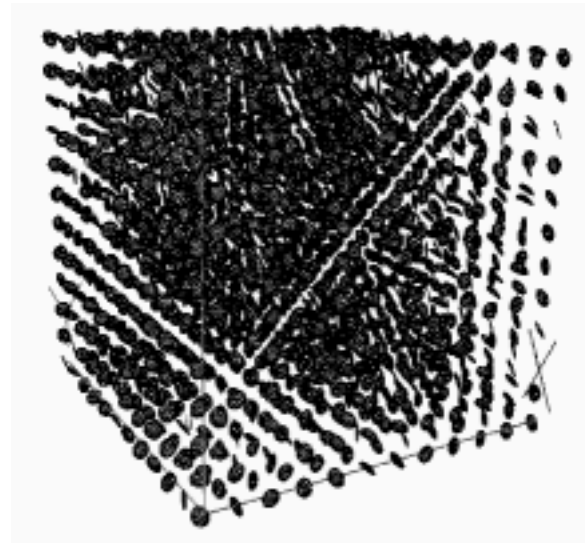
Fig. 4 crack opening displacement (DOF=1,285,632) of an array of 12 \times 12 \times 12 penny-shaped cracks
